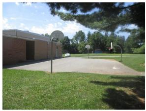
Rain gardens adjacent to the building can capture, treat, and infiltrate roof runoff. A water harvesting system such as a cistern can collect rainfall from rooftops as well and be put to other uses. The basketball court can be replaced with porous pavement to intercept and infiltrate rainwater from the rooftop as well as its surface. A preliminary soil assessment suggests that the soils have suitable drainage characteristics for green infrastructure.
