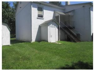
A rain garden adjacent to the building in the northwest corner can capture, treat, and infiltrate roof runoff. A preliminary soil assessment suggests that the soils have suitable drainage characteristics for green infrastructure.
