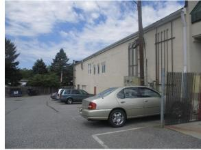
Parking spaces adjacent to the building can be replaced with porous asphalt to intercept stormwater runoff from the roof. A preliminary soil assessment suggests that the soils have suitable drainage characteristics for green infrastructure.
